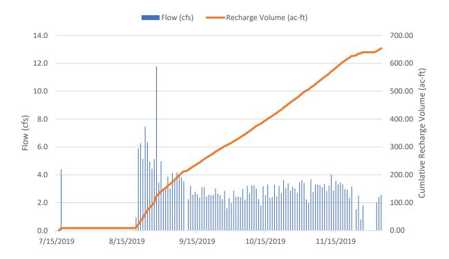
Figure 2-3: Demonstration Test Flow and Cumulative Recharge Volume
