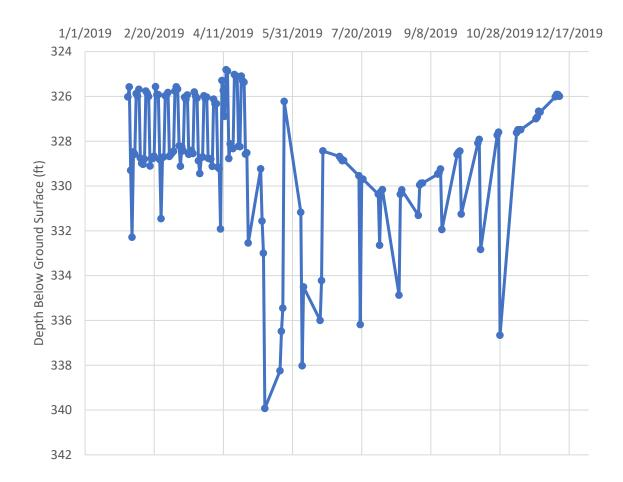
Figure 2-6: Groundwater Levels During Demonstration Test
