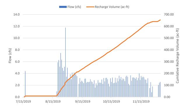
Figure 5: Demonstration Test Flow and Cumulative Recharge Volume
