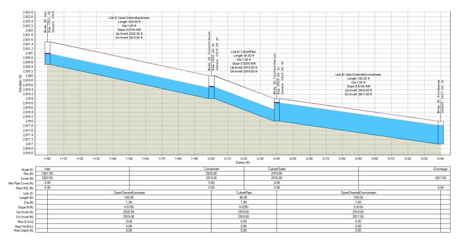
Figure 4-2: Box Culvert Hydraulic Profile
